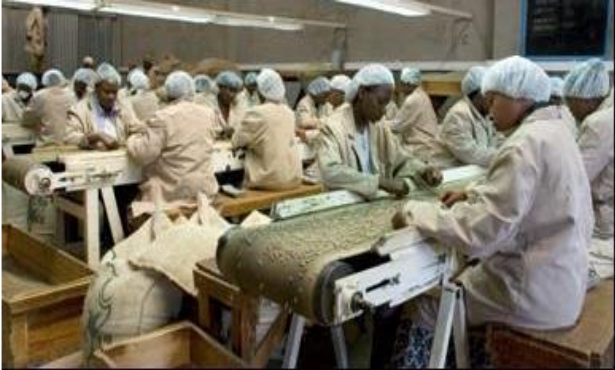
Figure 4.5: Manual sorting of green coffee on tables manned with conveyor belt
