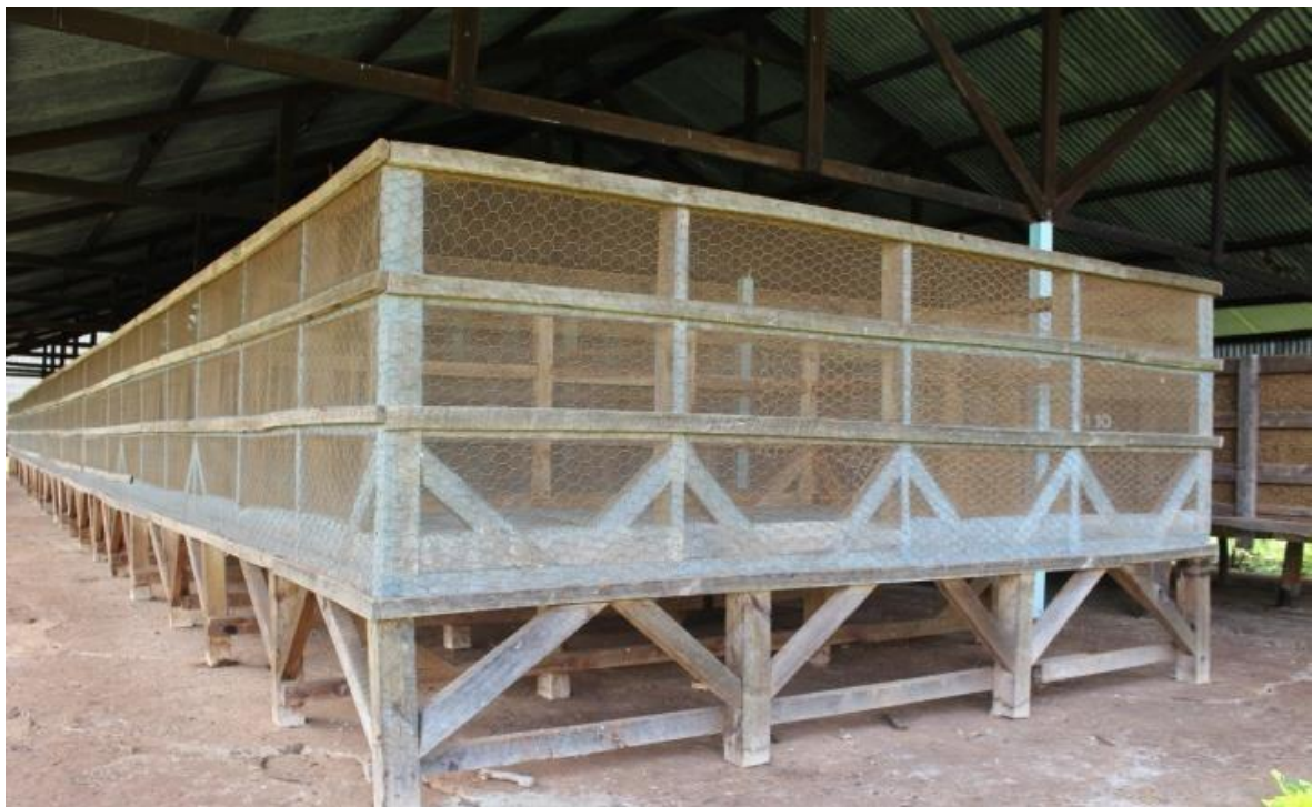
Figure 3.14: Conditioning bins for evening out moisture level
