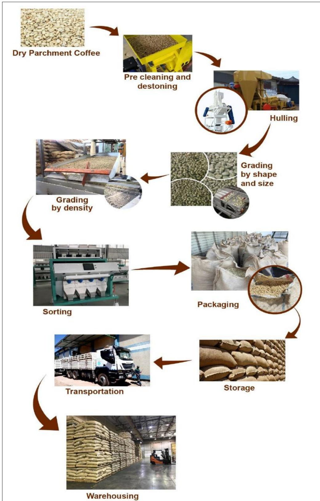
Figure 4.2: Diagrammatic presentation of secondary processing
