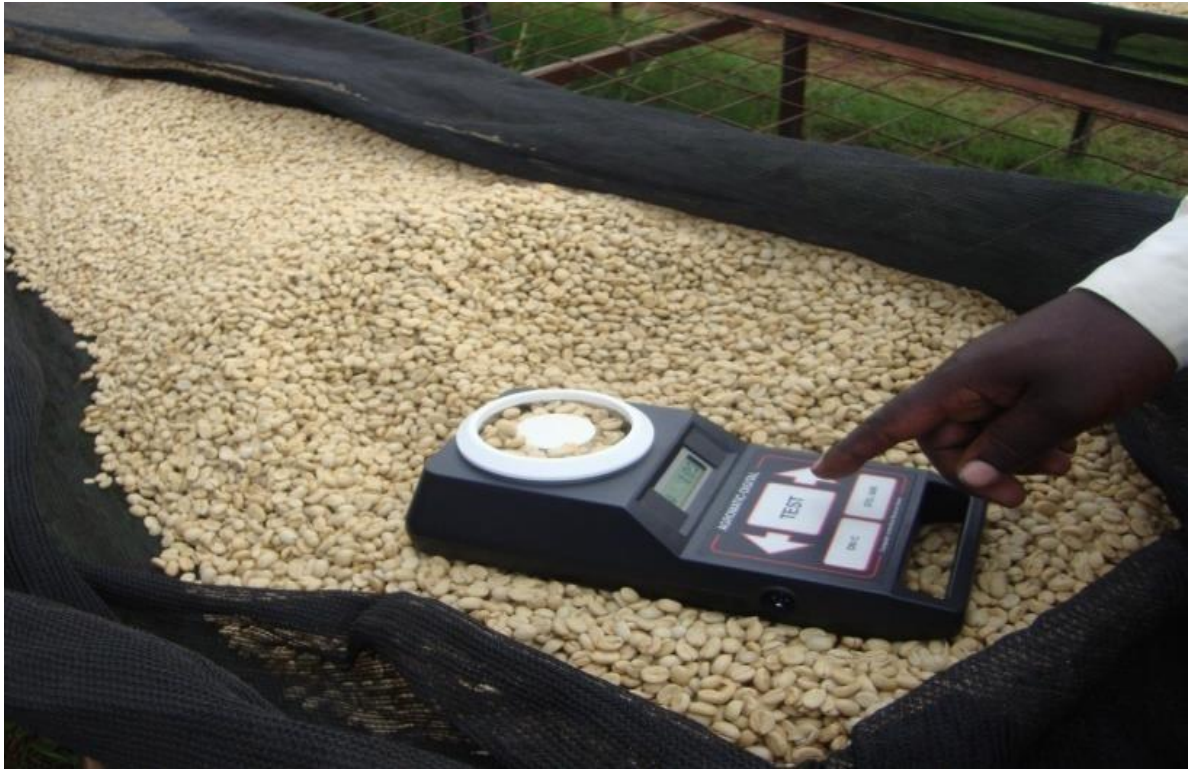
Figure 3.13: Testing of parchment moisture using a moisture meter
